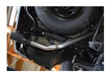
Install the Gibson Tips onto your exit pipes. Place the tips to your desired position. Be for tightening down the system it is recommended to secure the tips in the position you want and check the location after each connection is tightened.
