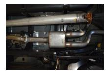
Install muffler onto head pipe # A 1-1/2" to 2". Use a jack stand to support the muffler. Use clamp #I to the secure the muffler to the head pipe. Do not tighten
